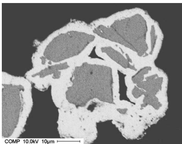
Figure 6 Back-scattered micrograph of agglomerate of particles coated at pH12.
